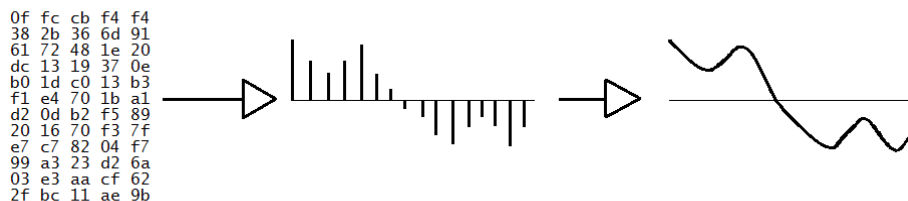
Figure 3. The pulse-code modulation stream to digital signal to analog signal chain
