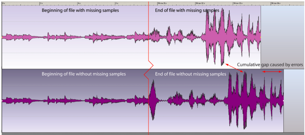
Figure 4: Demonstrating the beginning and end of the DAW and Reference files. Note that they are synchronized in the beginning and that by the end they are out of sync due to missing samples in the DAW file.
